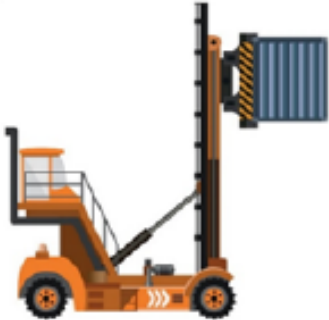
Large-scale port machinery (top handler)
